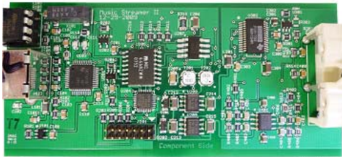
The HRT Music Streamer II features a Texas Instruments TAS1020B input transceiver running custom firmware (left), feeding a Burr Brown PCM1793 DAC (top right)
