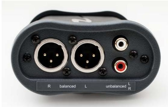
On the left side of the rear panel of the MSHD are two “balanced” XLR connectors, one labeled “R” and one labeled “L”. These correspond to the audio channels where “L” is for the Left channel and “R” is for the Right channel. The XLR connectors have a full scale output of 4.5 Volts RMS in level, so if you choose to use the balanced outputs, please make certain that your audio system is capable of properly handling the maximum level that the MSHD can output.
