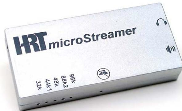
On the right hand side of the microStreamer you will find two 3.5mm sockets. These two sockets are for connection to either or both, headphones and your audio system. The two sockets, though similar in appearance have different characteristics optimized to their specific use.
